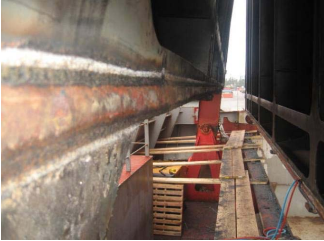
Rubber channel at aft part removed
