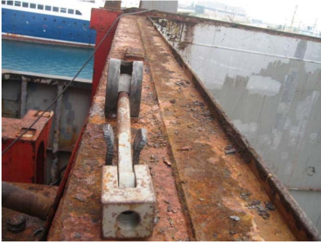
Reconditioned cleat with Fabricated onboard crutch
